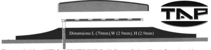
Piezo ceramic pickup (UST) for ACOUSTIC GUITAR with distance of strings (55mm). Every piezo pickup constructed with separate ceramic element's and skillfully assemble with great precision. That improving the balance between strings. Excellent frequency response characteristics and natural sound reproduction. Perfectly you can combine this with external preamplifier and also with ENJ preamplifier built-in on endpin jack.
